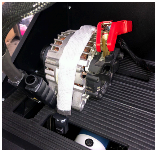
Figure 16. Connection of Power Wires to the Alternator
