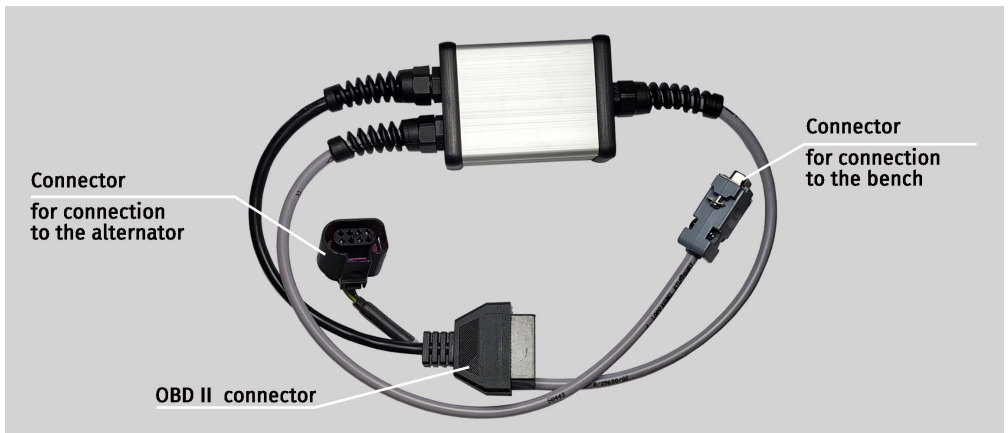
Figure 8. Cable for diagnostics of belt starter-generators 48 V AUDI
