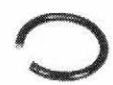
S-2156 Retainer Ring For Chrysler solenoid mounted (tin can type) .404" I.D. x .587" O.D. x .095" Thk.
