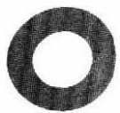
S-694 Fiber Washer For Chrysler solenoid mounted (tin can type) 5/8" I.D. x 1 1/4" O.D. x .043" Thk.
